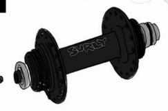
Our Ultra New hubs have shells made from 6061-T6 forged and machined aluminum with hollow 4130 CroMoly axles of our own design and 304 Stainless Steel fixing bolts. Ultra New hubs can be converted to QR by simply removing the bolts and installing a QR skewer. Our Ultra New hubs come in black or silver with pretty much any spacing, brake type (disc or non), or hole count you can imagine so head to surlybikes.com to get the full picture of all the hubs we offer.
