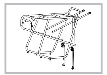
Frequently check to make sure that all of the rack hardware is properly torqued per these instructions. Check to make sure that the rack mounting bolts are properly tightened and secure the rack to the bicycle frame. Periodically check for any signs of cracking or failure and discontinue use if rack is damaged.
