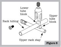
7. Install upper barrels onto the rack tube
